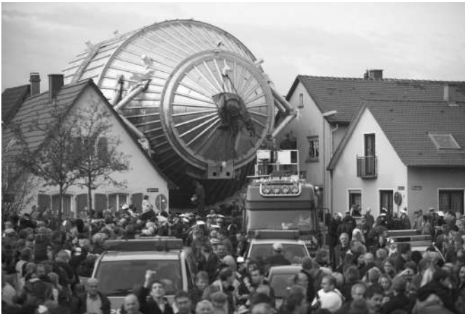
Figure 6.8. Transport of the spectrometer towards its final destination at Karlsruhe. With kind permission of the KIT and the KATRIN collaboration.
