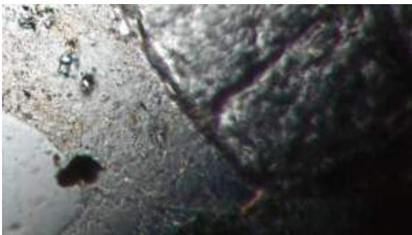
Figure 2.5.3A. Accessory plate partially obscuring the view of a thin section.
