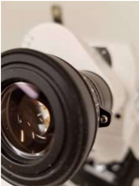
Figure 2.5.2A. Eyepiece oriented with crosshairs horizontal/vertical.
