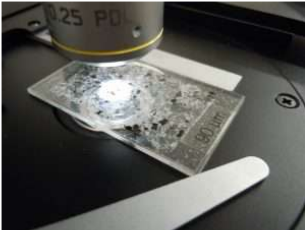
Figure 2.5.4A. A thin section right side up on the stage. Note you can see the edge of the cover slip and top layer of epoxy all the way around the top edge of the thin section.
