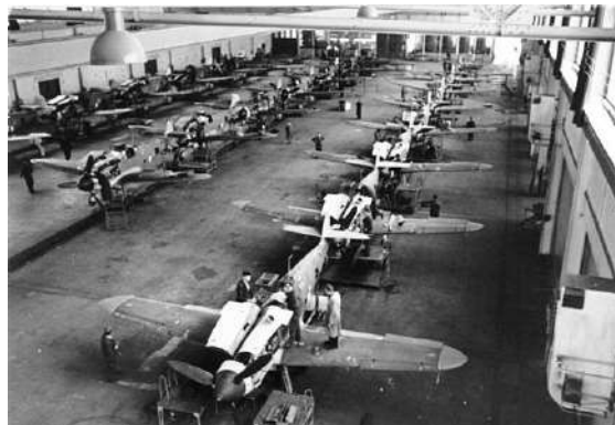
Assembly line of Messerschmitt Bf 109G-6s fighters in a German aircraft factory.
