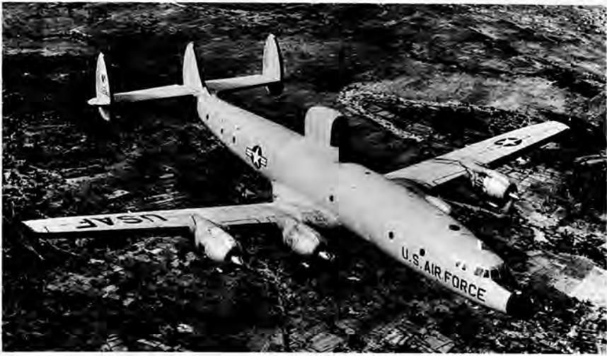
USAF EC-121 early warning radar surveillance aircraft in flight over South Vietnam.
