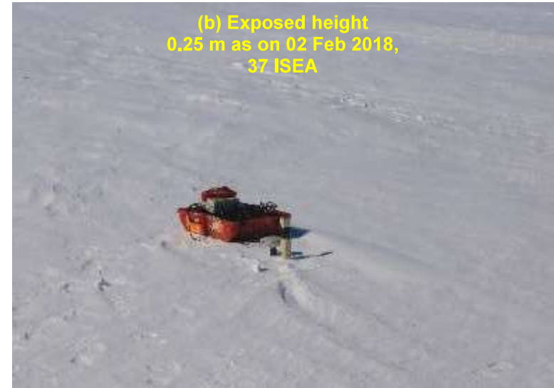
Figure 4.21: Field photo of DGPS measurement on feeder ice sheet of Polar Record Glacier installed bamboo log (a) exposed (a) exposed height 1.24 m as on 14 Jan 2017(36 ISEA) (b) exposed height 0.25 m as on 02 Feb 2018 (37 ISEA).
