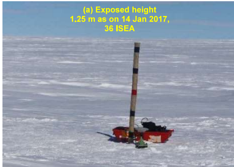
Figure 4.21: Field photo of DGPS measurement on feeder ice sheet of Polar Record Glacier installed bamboo log (a) exposed (a) exposed height 1.24 m as on 14 Jan 2017(36 ISEA) (b) exposed height 0.25 m as on 02 Feb 2018 (37 ISEA).
