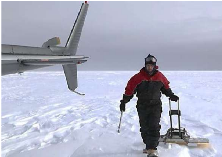
Figure 4.15: GPR observation on iceberg UK235 during 35 th ISEA.
